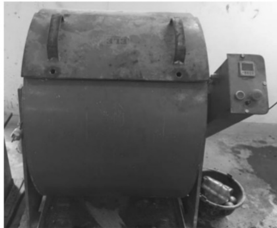
Fig. 2 Los Angeles machine for abrasion test
